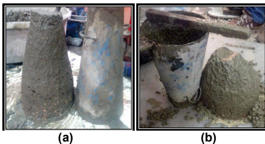
Fig. 6. Slump test; concrete a) without Superplasticizer, b) with Superplasticizer
