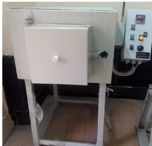
Fig. 2. Oven carry up to 1200°C
